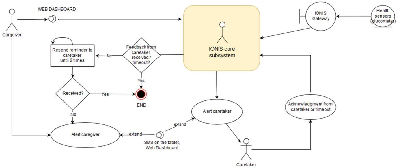
**Figure 13. UML diagram for the reminder and alerts use-case.**
