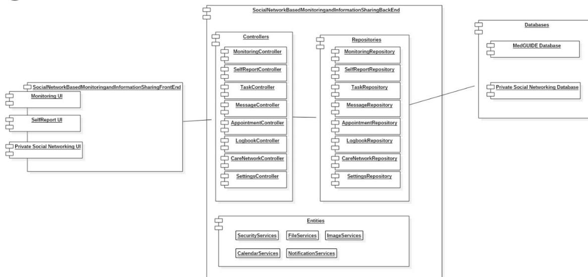
**Figure 27 UML component diagram illustrating the development view of the Social network-based monitoring and information sharing service**
