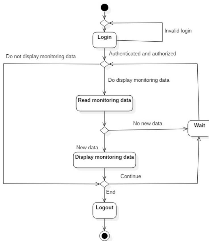
**Figure 25 UML activity diagram illustrating the flow of the Monitoring process**
