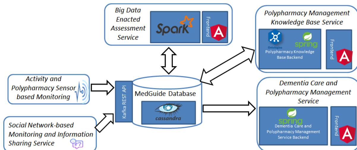
**Figure 18 MedGuide system overall architecture**
