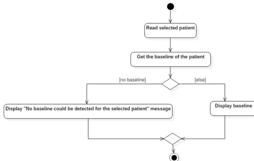
**Figure 31 UML activity diagram illustrating the flow of the Baseline Detection and Visualization process**
