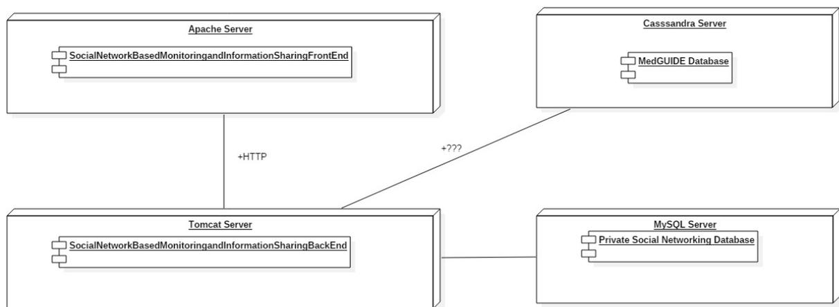
**Figure 28 Deployment architecture for Social network-based monitoring and information sharing subsystem**
