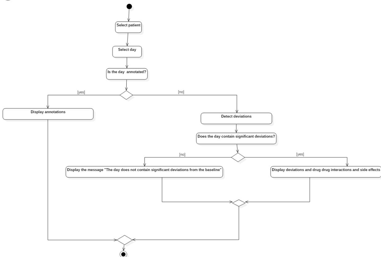
Figure 32 UML activity diagram illustrating the flow of the Deviations Detection process
