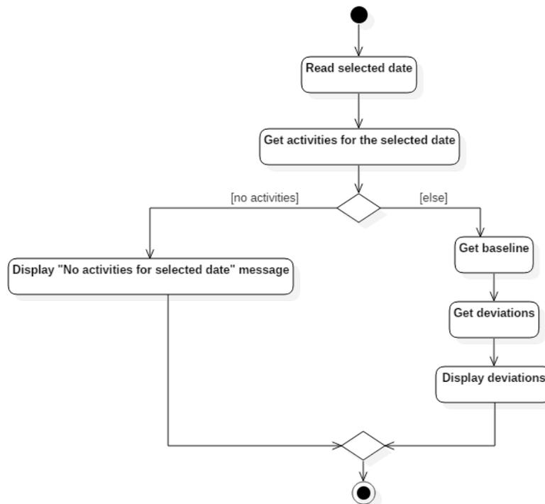
**Figure 37 UML activity diagram illustrating the flow of the Baseline and Deviations Visualisation process**
