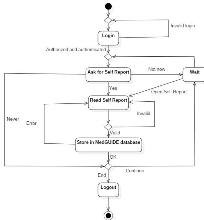
**Figure 24 UML activity diagram illustrating the flow of the Self Reports process**
