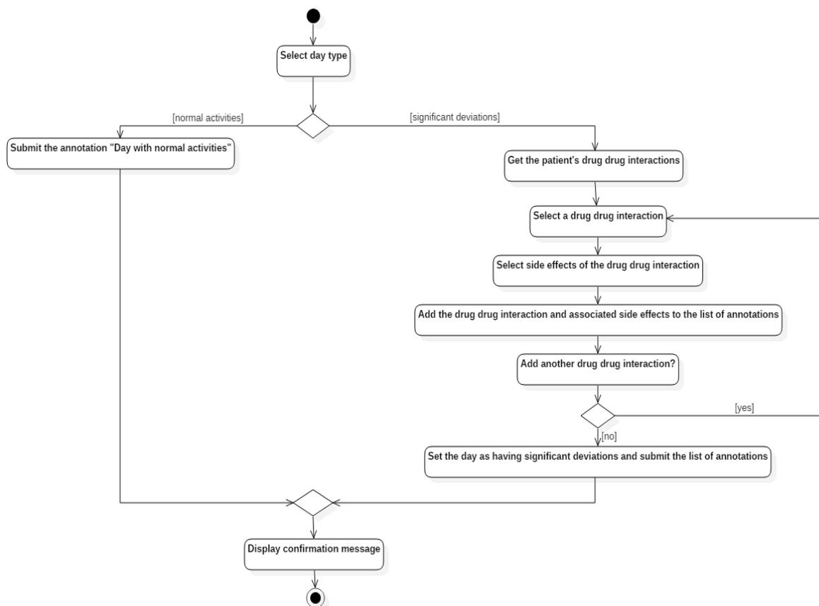
**Figure 38 UML activity diagram illustrating the flow of the Deviations Annotation process**
