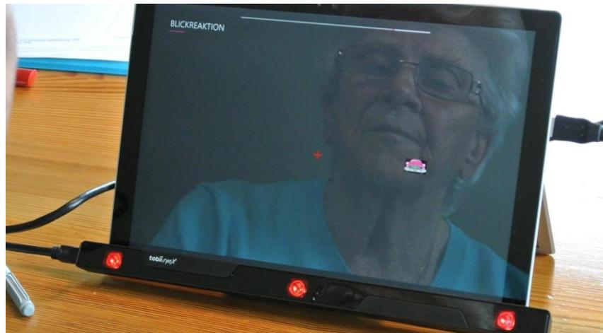
*Figure 1. Eye tracking (mobile interface attached at the bottom of the tablet PC) applied to an Anti-Saccadic task for the assessment of cognitive control.*
