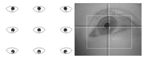
Figure 2. The relationship between the pupil center and the corneal reflection when the user fixates on different locations on the screen (Adapted from Majaranta et al. 2009b)
