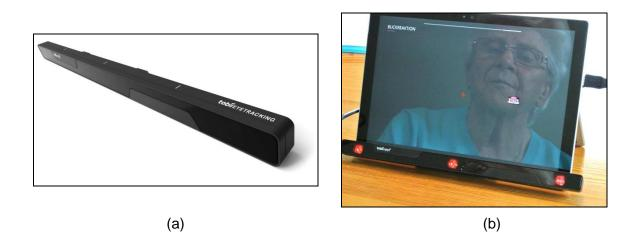
Figure 4. Mobile eye tracker solution Tobii EyeX. (a) The mobile eye tracking device is easily attaches to tablet PCs. (b) The mobile eye tracking device in operation while a person with dementia is performing a playful cognitive control task.
