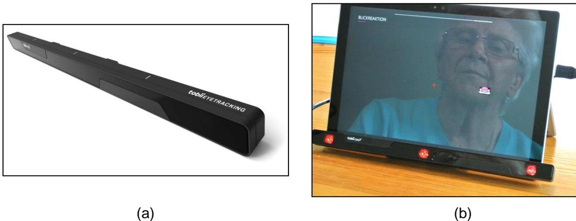
Figure 4. Mobile eye tracker solution Tobii EyeX. (a) The mobile eye tracking device is easily attaches to tablet PCs. (b) The mobile eye tracking device in operation while a person with dementia is performing a playful cognitive control task.
