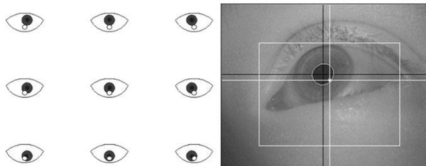
*Figure 2. The relationship between the pupil center and the corneal reflection when the user fixates on different locations on the screen (Adapted from Majaranta et al. 2009b)*
