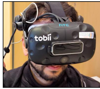
Figure 4: For the study a HTC Vive head-mounted device with built-in eye tracking from Tobii and Leap Motion sensor was used.
