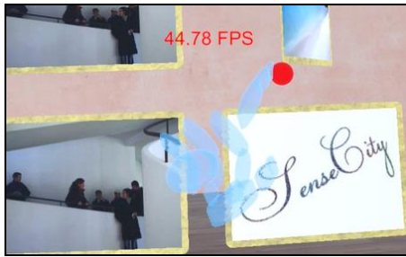
Figure 3: Hand gesture (Leap Motion) for the selection of affectively weighted image ‘cards’.
