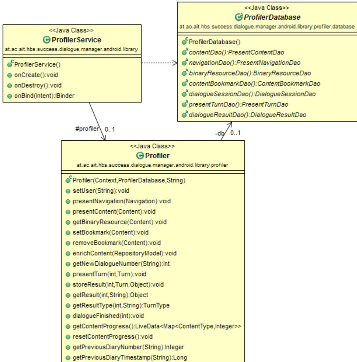
Figure 9: Profiler database implementation
