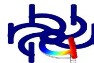
Figure 3: Eigenmode simulation of the monolithic structure with a first resonant frequency around 100 Hz.
