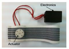
Figure 1: Tactile bracelet with six actuators placed on a wristband
