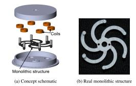
Figure 2: Monolithic structure with six lever beams and stimulators at each extremity
