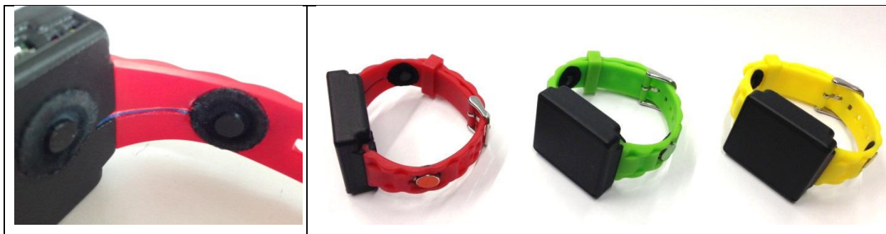
Figure 8: Flexible membranes of the 4 th version (left) and 3 prototypes (right)
