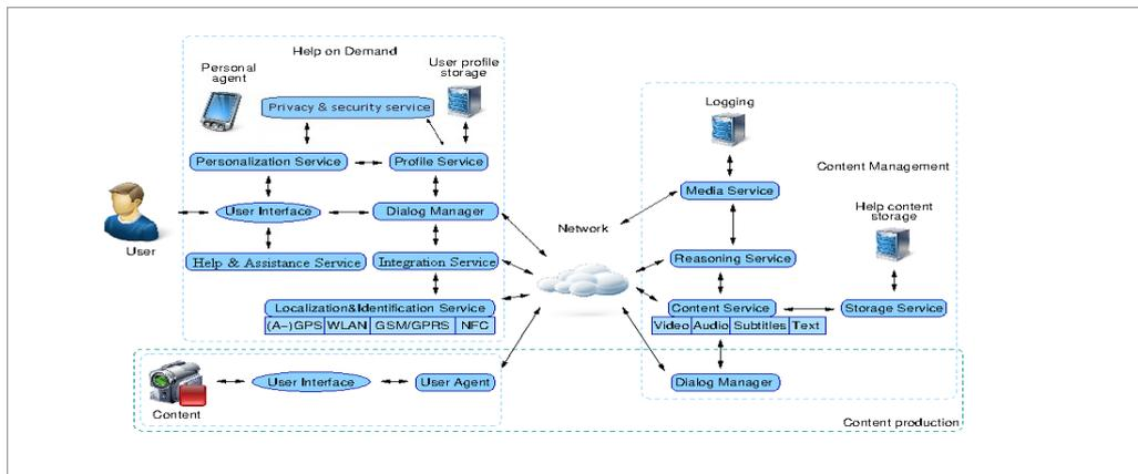
Figure 1 System Architecture for Help on Demand Service
