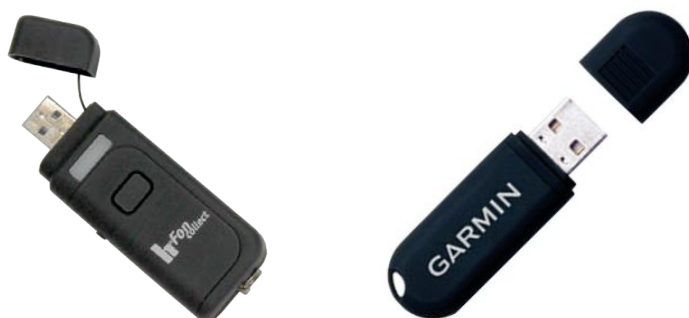
Figure 35: Mobile gateway HMM hFon Collect (left) and software gateway ANT+ dongle (right)
