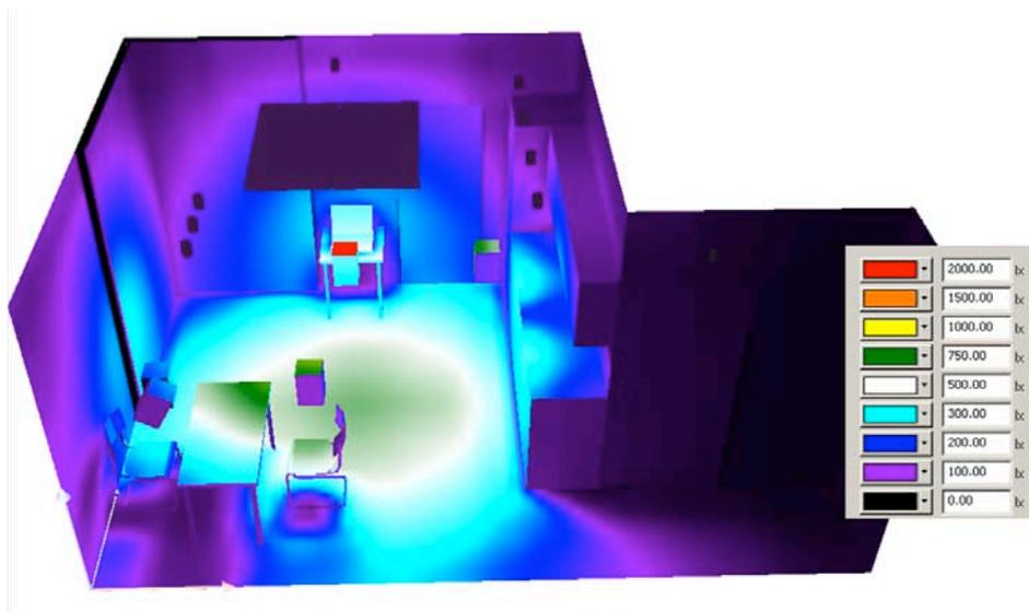
**Fig. 11 False color visualization for the situation ambient light with light field**
