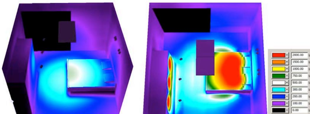
**Fig. 12 False color comparison of different lighting situation within the sleeping room with light fields**
