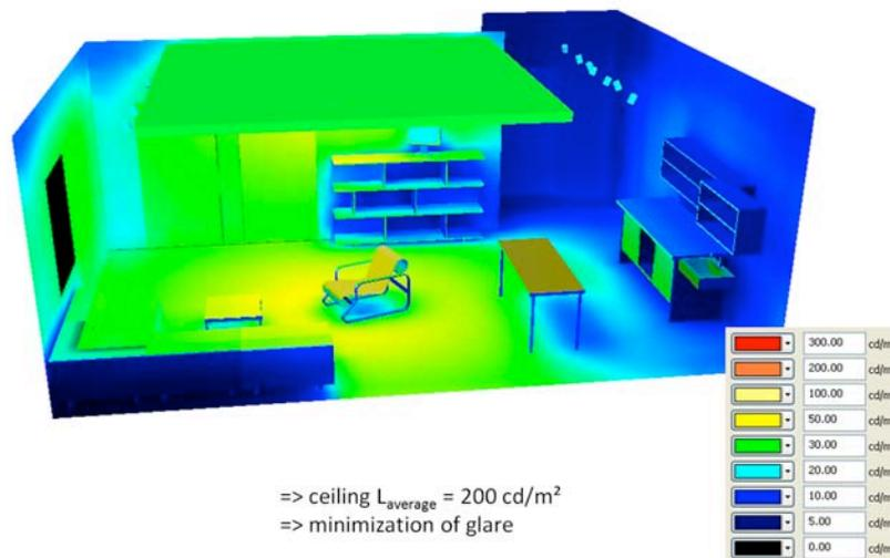
**Fig. 1 False color visualization of the ambient light situation**
