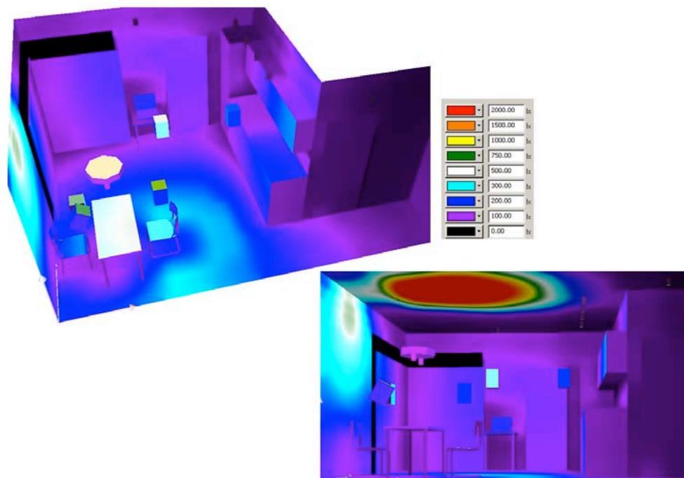
**Fig. 8 False color visualization for the situation ambient light with a suspended luminaire**
