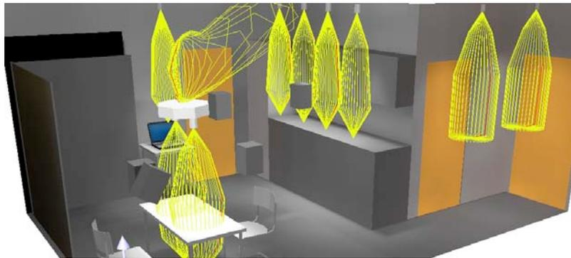
**Fig. 9 Schematic visualization of the light intensity distribution of the luminaires**
