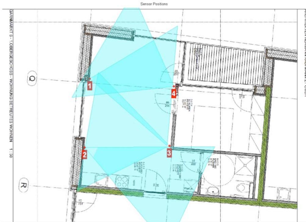
Fig. 22 Single room coverage by an optical system (example: Intenta)
