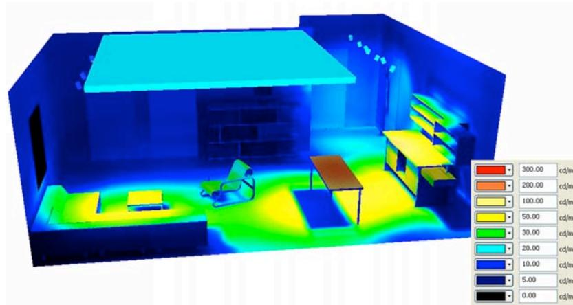
**Fig. 2 False color visualization of a zonally task light situation**
