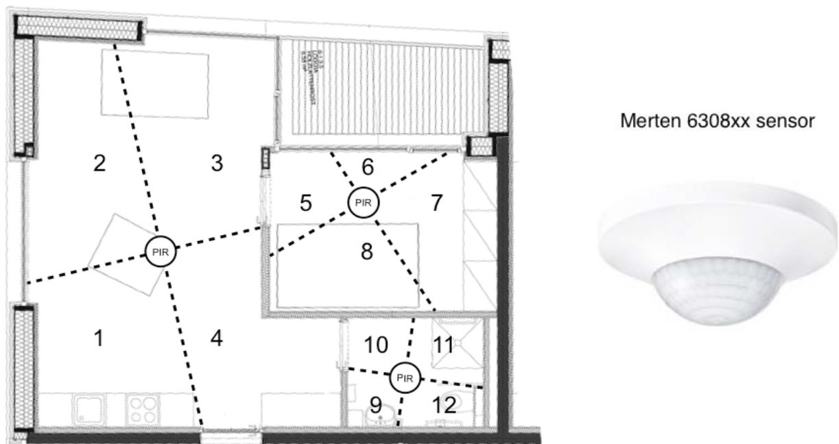
Fig. 24 Plan of test apartment with numbered PIR-sensor sections (total 12 sections).
