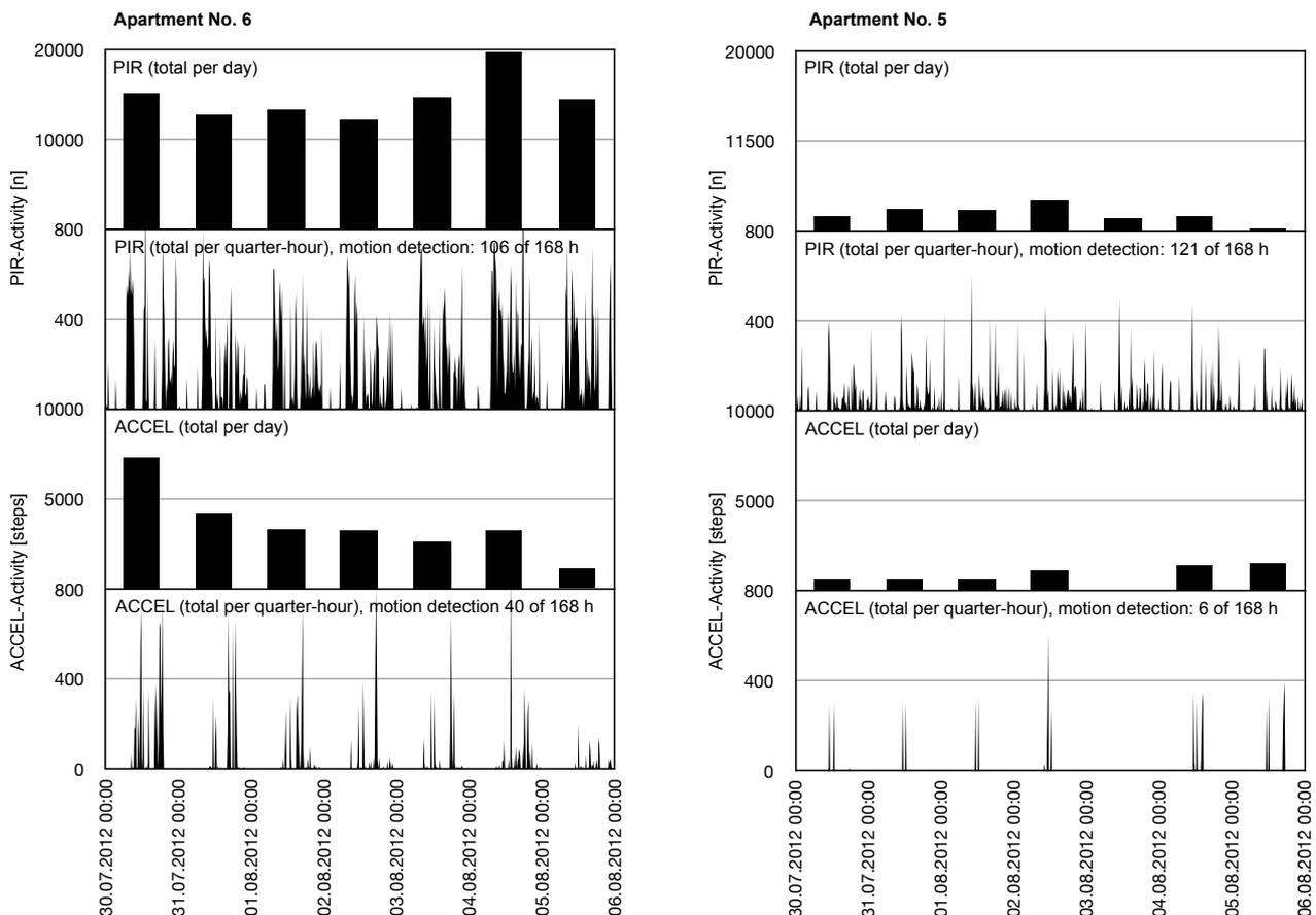
**Fig. 17 Comparison of data quality of PIR sensors and actigraph.**
