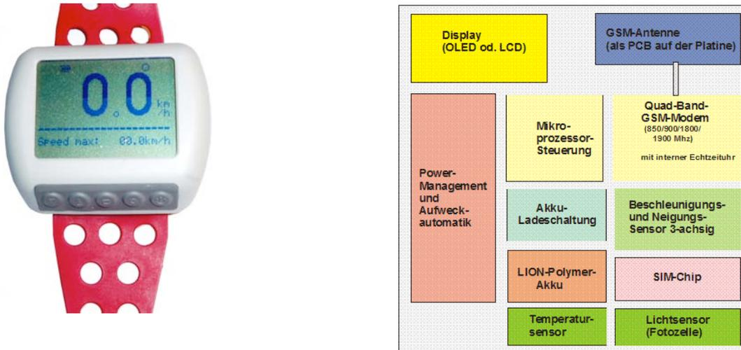
Fig. 30 Example of an individual sensor device and the components (source: Fidelak)
