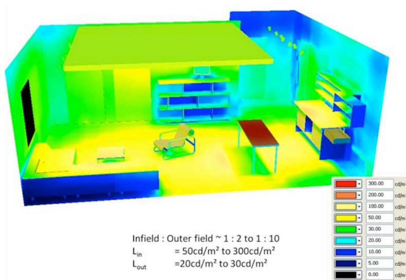
**Fig. 3 False color visualization for the situation “all luminaires switched on”**
