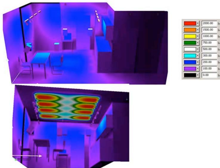
**Fig. 7 False color visualization for the situation ambient light with ceiling washer**
