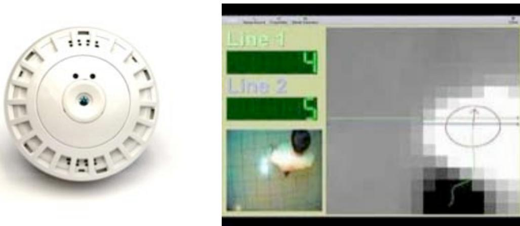
Fig. 23 Thermal sensor array Irisys IRC3010 IP.
