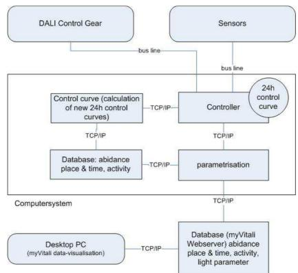
Fig. 2 System architecture for a wired lighting control solution
