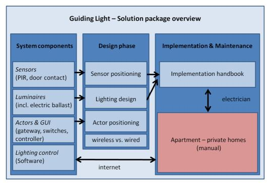
Fig. 1 Integrated overview of the GL-system
