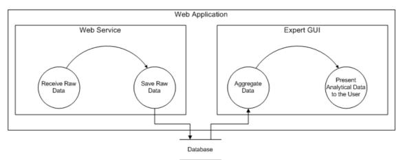
Fig. 25 Data flow diagram of the Web Application (Expert GUI)
