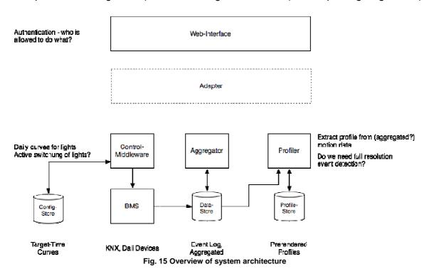
Within data management layer we retrieve all event log information from building management system and will provide data aggregation. Aggregator will select all relevant information from BMS and transfer them to the unified data structure described in the chapter User monitoring with one data line per minute. A profiler will extract user profiles from aggregated motion data and will store pre-rendered profiles in a profile store.
