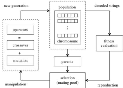
Fig. 22 Process flow diagram of automatic lighting control by means of genetic algorithm
