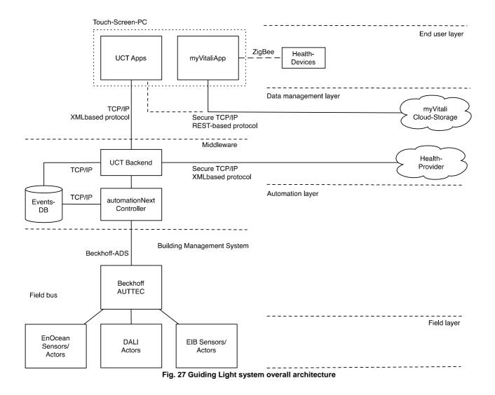
We are developing middleware software for automation layer to retrieve all event log information from building management system and to transfer daily control signal curve for lights, active switching of lights (time controlled or in relation to presence and light level) from our config store over TCP/IP connections.
