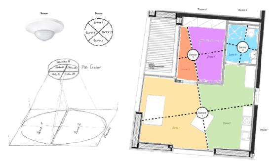
Fig. 16 Assignment of sectors of motion sensors to room zones
