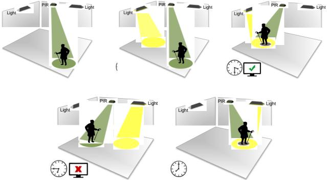
Fig. 11 Main principle of zonally lighting within lighting control strategy 2
