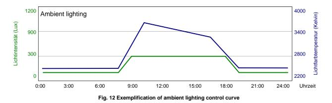
If we would cumulate all zonally light signal curves we would receive a more accentuated ambient light signal curve. Each luminaire can be manually turned off or on by inhabitant.
