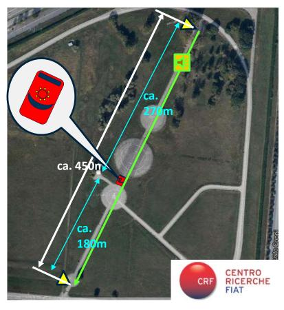
Localization result (DSB) without additive noise, frequency range: 600Hz – 4kHz
