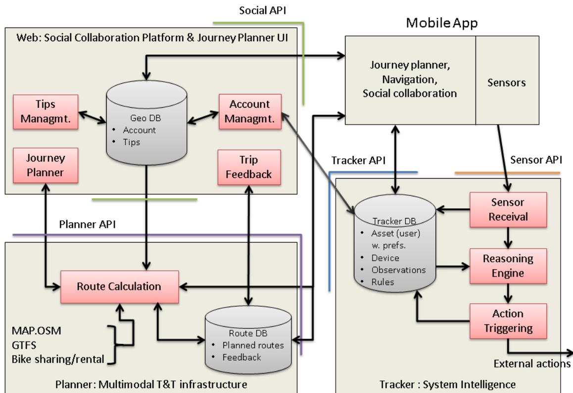
Figure 9: Logical view of T&Tnet system
