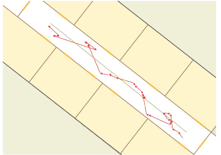
Fig. 4. Real trajectory (grey straight line segments) and path from position estimations (red crooked line segments).
