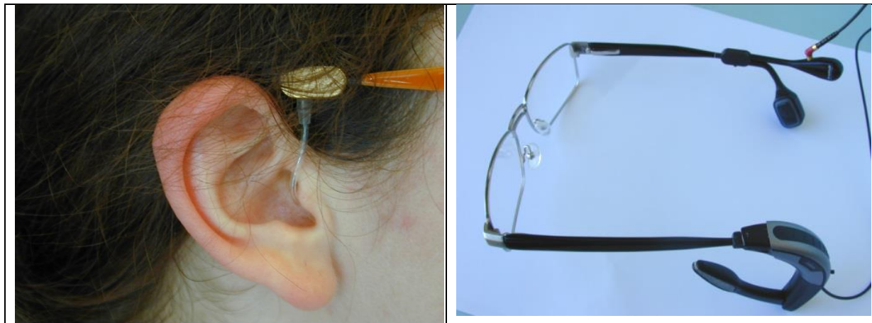
Figure 3. Hearing aid glasses with the in-ear hearing device, left and with the Cossinus prototype and bone conduction speaker. The glasses will include also micro for seamless voice interaction.
