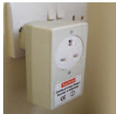
Figure 8: Electrical Usage sensor
