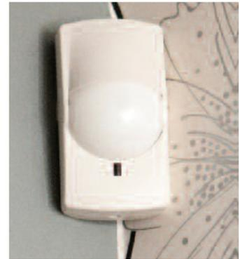
Figure 9: Motion Detection sensor
