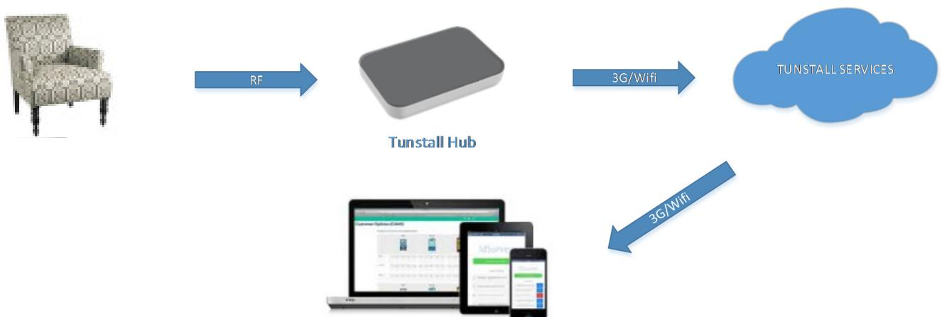
Figure10: Environmental Sensor Example
