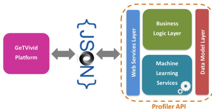
Figure 4: Current Profiler Architecture
