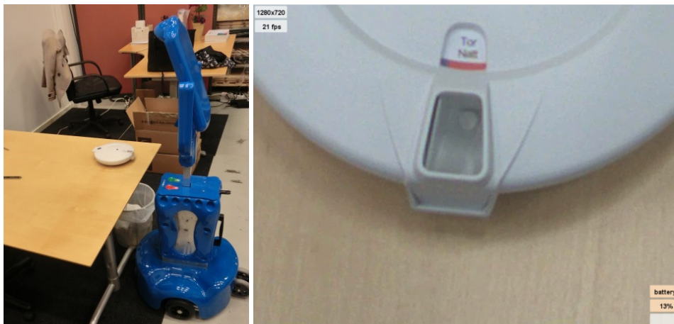
Figure 5: The Giraff zoom capability. The left image is of the Giraff side, the right is from the Pilot application.
