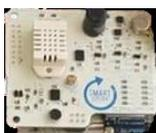
The environmental sensor (Urban Board) that measures indoor temperature, humidity, light, sound, carbon monoxide and nitrogen dioxide data among others, will be used to track the position of the user at any time in specific locations.
