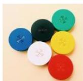
The BLE tags are placed in the environment of the user to identify the user's indoor location at any time.
