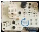
The environmental sensor (Urban Board) that measures indoor temperature, humidity, light, sound, carbon monoxide and nitrogen dioxide data among others, will be used to track the position of the user at any time in specific locations.
