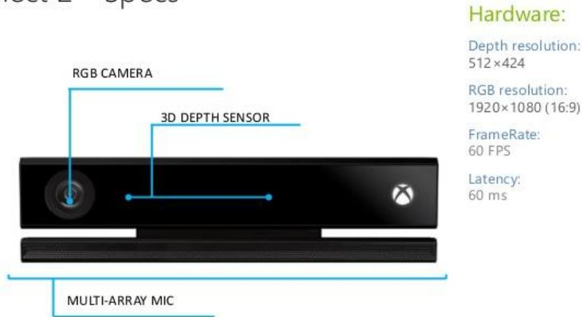
Figure 2.5 . Kinect 2 sensor
