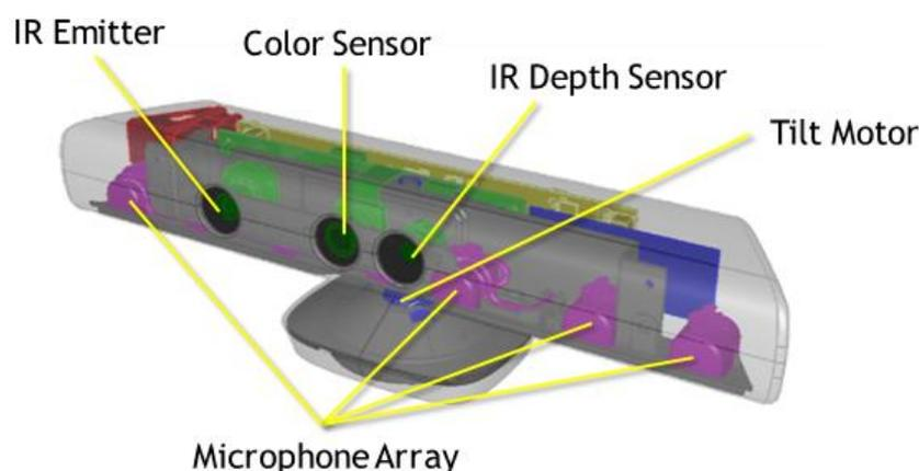
Figure 2.4 . Kinect sensor
