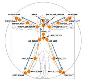
Figure 3.3 . Common body joints detected by skeleton tracking libraries
