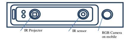
Figure 2.3 . Hardware Diagram for the Structure Sensor device
