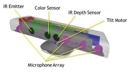
Figure 2.4 . Kinect sensor
