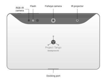
Figure 2.2 . Hardware Diagram for the Tango Tablet Development Kit
