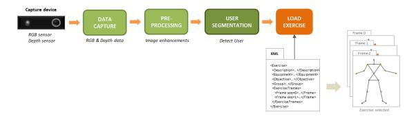
Figure 3.4 . Functional blocks of the 3D Motion Sensing module (I)
