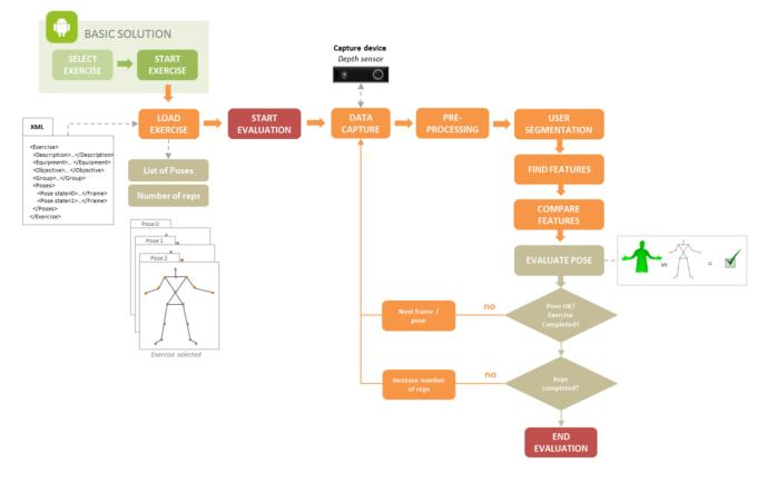
Figure 3.2 . Functioning of the 3D Motion Sensing module
