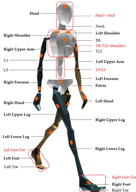
Figure 5.1 The location of the sensors and the tracked parts of the body [KinematicModel]
