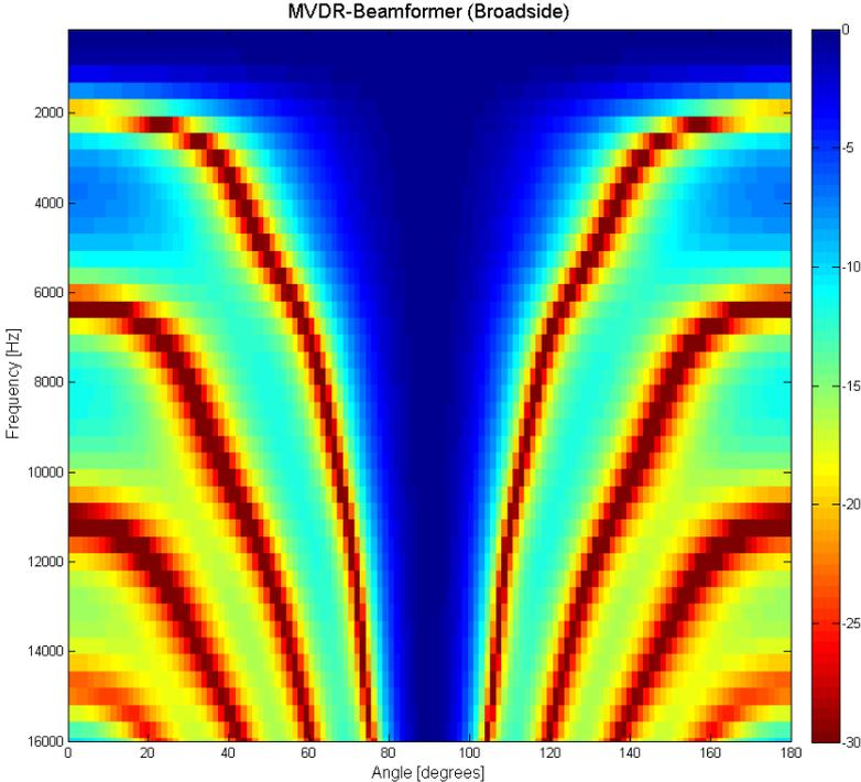
Figure 6: Beam pattern of array simulation for different angles and frequencies.
