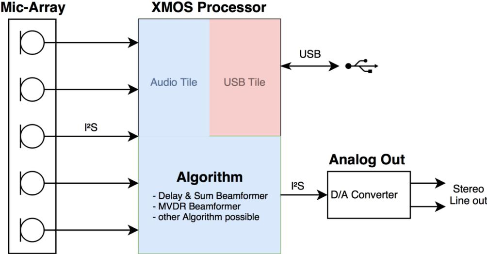
Figure 5: Audio Processing Unit (signal flow graph)
