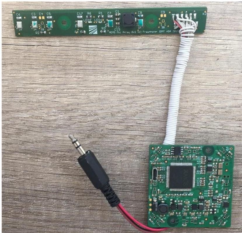
Figure 4: Audio processing unit (microphone array (upper part) and signal processing unit (lower part))
