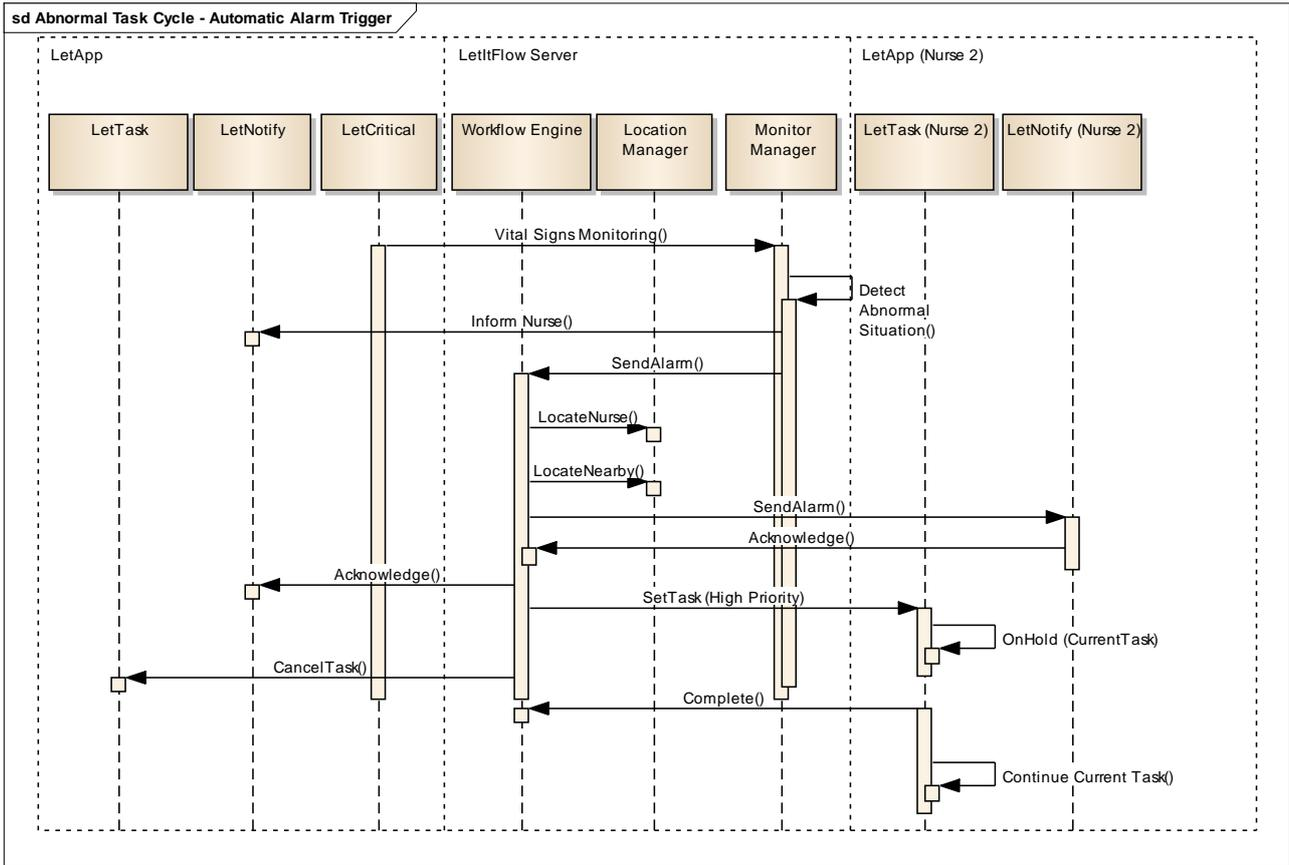
Figure 17 Automatic Alarm Trigger
