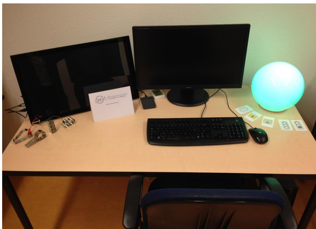
Figure 4. Technological setup for the field trials of PEARL, consisting a desktop PC, a second screen (touch based), a keyboard, a mouse, a RFID-reader, a RFID-card (to login), an availability indicator, an ambient light, and a digital-analogue calendar.
