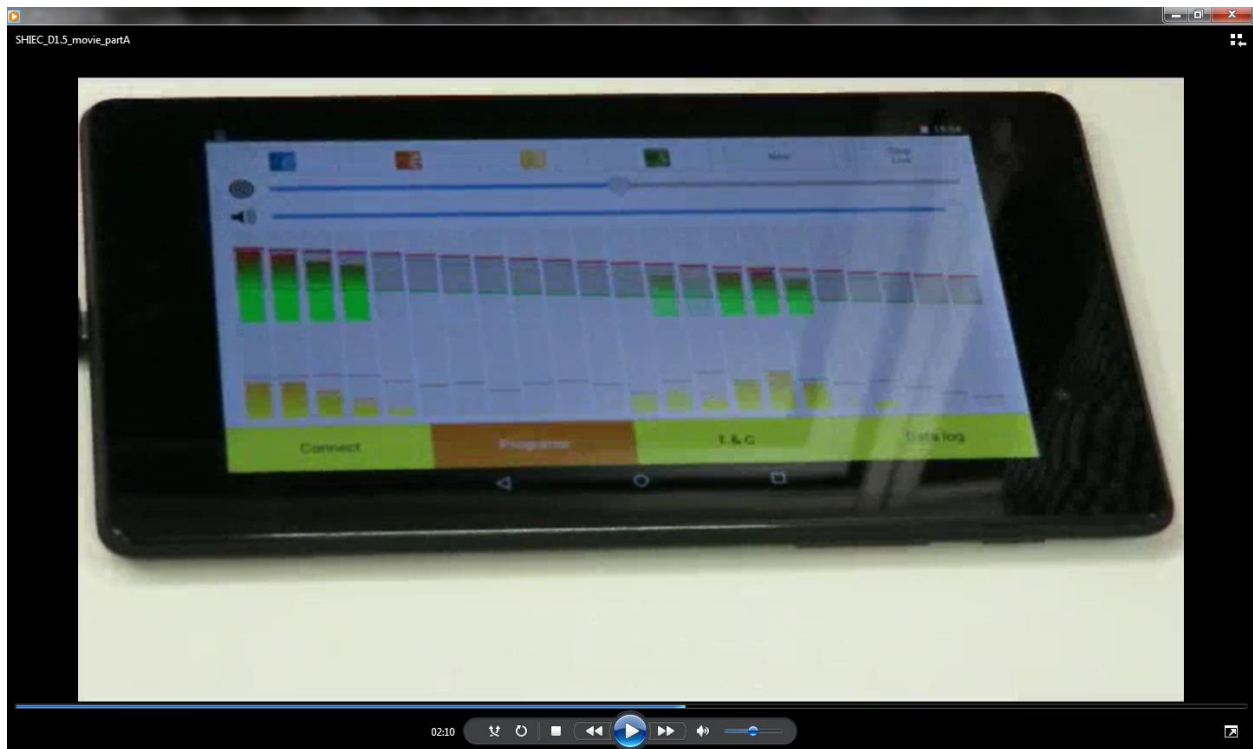
Figure 2: movie demonstrating a real-time connection from a tablet computer (Android) to the sound processor. The application is a clinician application (fitting the device parameters for a particular patient).
