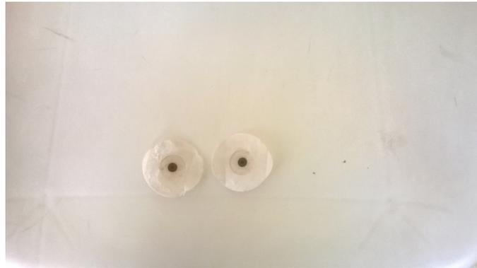
The electrodes with conductive gel have to be put on fingertips of index and medium fingers. The subject has to hold the device in his palm.
